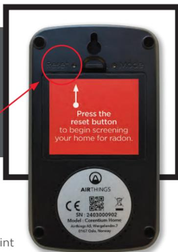
*We recommend you do not press the mode button. It is only used to repair the device.*
