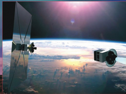
A solar sail propels a spacecraft because photons from the sun transfer their momentum to the ultralight sail.
