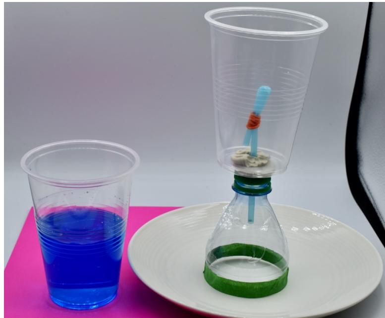
10. The cup will fill up until the level of the water reaches above the top of the straw. When it does most of the water will leak out. Test and Tweak.
