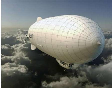
Unlike a balloon, a blimp has a shape and structure that enable it to fly and maneuver. The main part of a blimp is called the envelope. The envelope is the large bag that holds the gas, in this case, helium. The envelope is generally cigar-shaped, for aerodynamic purposes, and made of a durable airtight, lightweight fabric that is much like the fabric of a space suit. Since blimps are comparably light, they are much more fuel efficient than jets and other aircraft.
