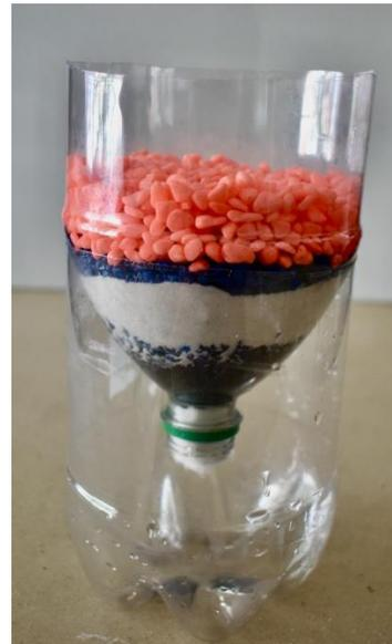
6. Finally, add the small pebbles. Make sure you completely cover the top of the gravel. See how the gaps between the particles of each layer have grown bigger and bigger toward the top. Now that your water filter is ready to put to work, you need to make some dirty water.
