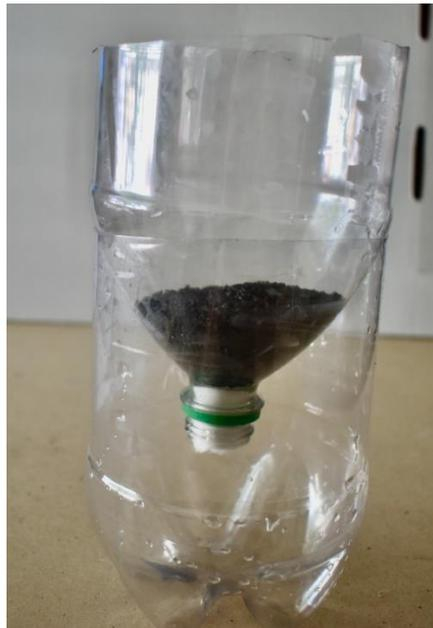
4. Add sand about 2 cm deep. Press it hard with your fingertips to push down the sand and the charcoal beneath it. These packed layers will slow down the water flow, trapping lots of dirt.
