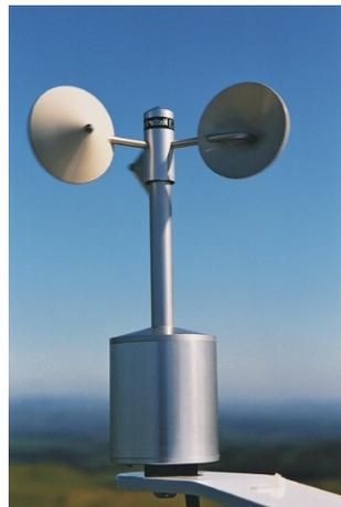
Find out how to read the wind! The only difference between a howling gale and a gentle breeze is how fast the air is moving. Meteorologists, the people who study weather, use a device called an anemometer to measure wind speed. You can make one of these yourself and then broadcast weather reports to your family.
