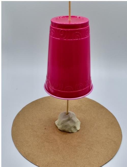
6. Slip the open end of the straw over the skewer. If your wind-catching cups won't stay level, fix them to the skewers with more adhesive putty. Finally, mark a dot on one cup, using the colouring tape. This lets you count every turn as the anemometer spins around. Go outside and test it.
