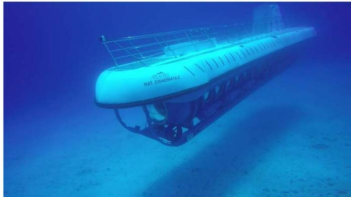
Submarines can change their buoyancy – that is how they rise to the surface and dive deep. They have tanks that can be filled with water or air. At the surface, they take water into these tanks, increasing their density – so they sink. To rise up, air is pumped into the tanks, reducing their density and allowing them to float to the surface.
