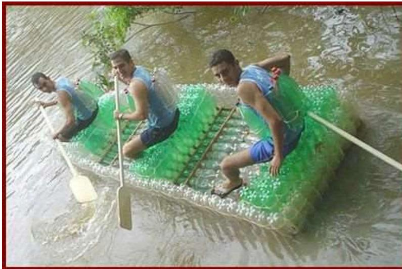
This activity could save your life! If you were stranded on a desert island and you had some large empty barrels, you could make a raft to escape. It is a simple matter of balancing forces. The weight on the raft's platform pushes the raft downward into the water, but this force is balanced out by the buoyance, or "up thrust," of the water pressing against the air-filled plastic bottles. Because these forces are equal, the raft floats.
