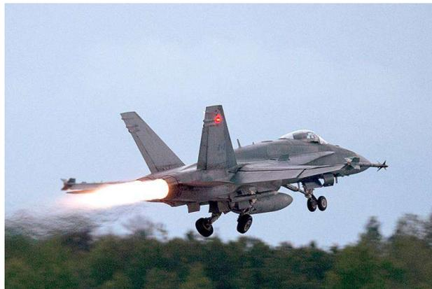
In a jet engine, spinning turbine blades draw in air. Heating and compression form hot gas that escapes through the exhaust nozzle of the aircraft. As this gas shoots backward, it pushes the aircraft forward at high speed.
