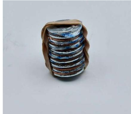
6. Attach one crocodile clip wire to each end of your battery, using the rubber band to hold everything in place. Make sure that the stripped wire ends are tucked firmly under the rubber band touching the metal on each end.
