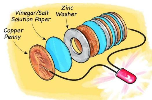
We use batteries to power many small devices – but how do they produce electric current? There is no better way to understand how batteries work than to build your own. In this project, you will build a battery made of coins, washers, and pieces of dishcloth – and use it to power a set of fairy lights.
